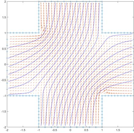
**Figure 1.** 2D potential flow model within the intersection of streets, based on the panel method.
