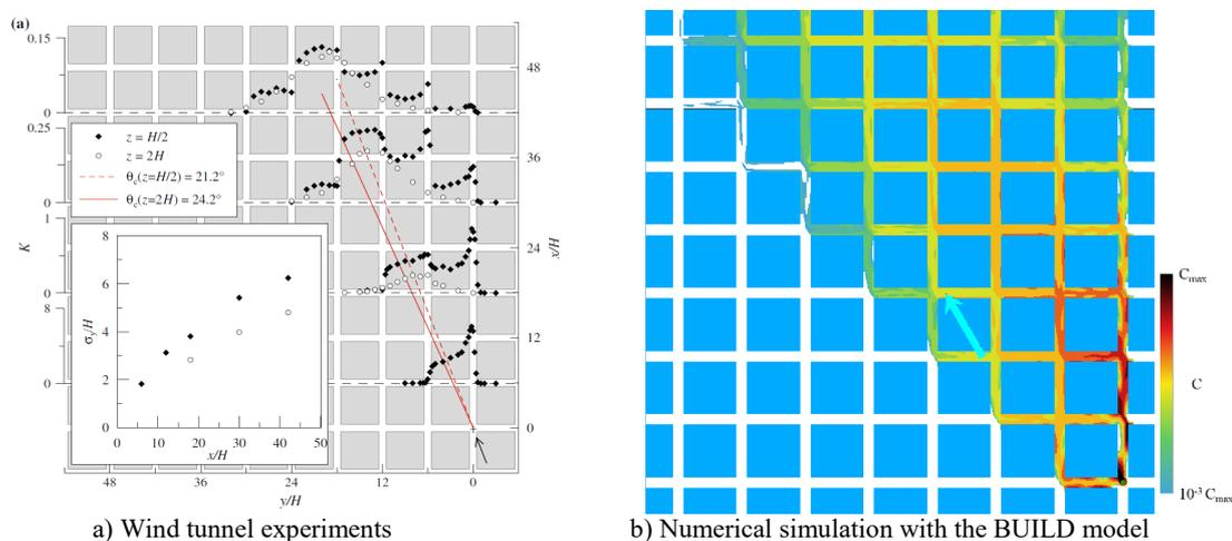
**Figure 4.** Concentration field in a network of streets for a wind direction  $\phi = 27.5^\circ$ : a) wind tunnel measurements and b) Numerical simulation with the BUILD model.
