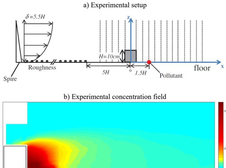
**Figure 3.** Experimental test case of the dispersion downwind of a two-dimensional square obstacle. The line source is located 1 H from the downwind wall of the obstacle.
