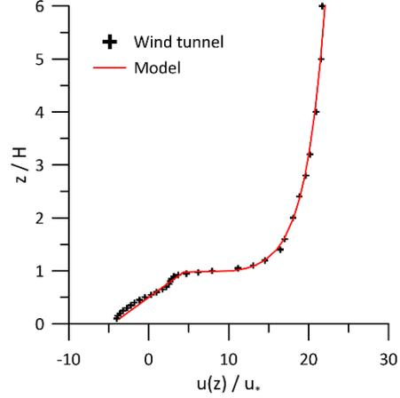
**Figure 2.** Vertical profile of the horizontal transverse component of the velocity inside and above a square street-canyon. Comparison between the analytical model and the wind tunnel experiments (Soulhac, 2000).
